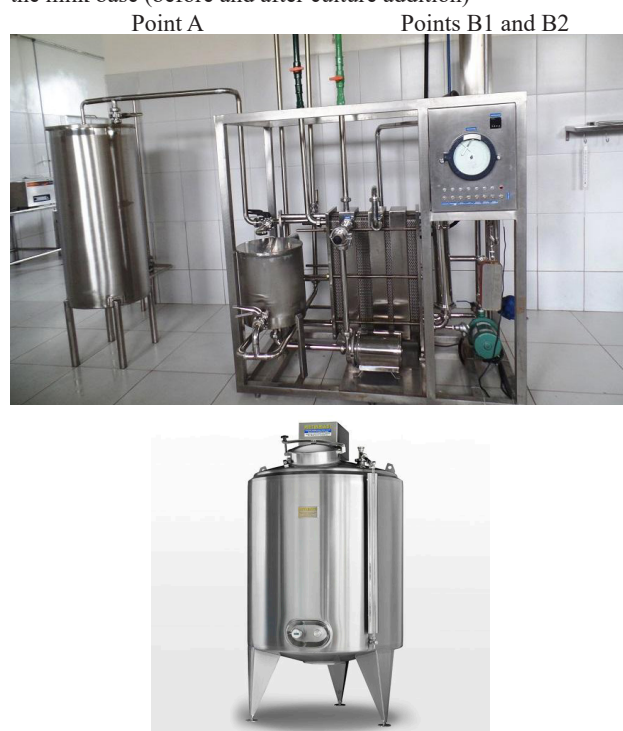
Figure 1 - Sampling points of the fermented dairy production line: Point A: milk base pasteurizer; Point B: fermentation tank of the milk base (before and after culture addition)
